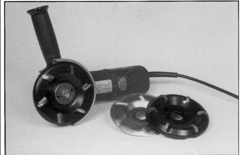
Carbide and steel wheel discs used to trim and shape hooves, woods and plastics.
