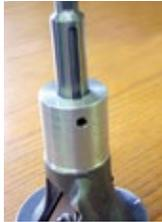
All the tenon cutters have an adjustable shaft to allow custom sizing of the length of the tenons. See chart for maximum tenon lengths.
