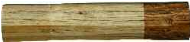
Prep Method used was Power Washing followed by a 3M™ non-woven pad.
