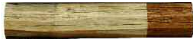
Prep method used was power washing followed by an Osborn Brush. The bare wood shown in the middle DOESN'T return to its natural color after pressure washing.
