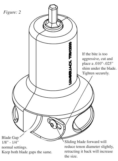
NOTE: *Do Not* slide it back more than 1/4" or it will not cut. Cutting green or dry logs and the species or type of wood (hardwood or softwood) will have an impact on power requirements. It will also affect the tenon size. Adjust tenon size to fit your requirements.
