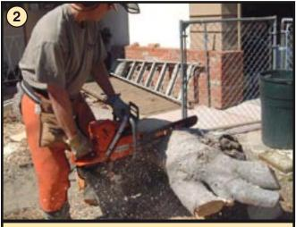
Trim the log to the length necessary to fit your first cut guide system.
