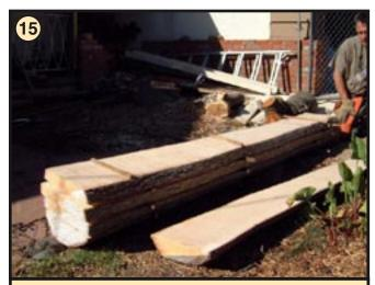
Stack cut slabs and place small stickers of about the same length and thickness between each slab.
