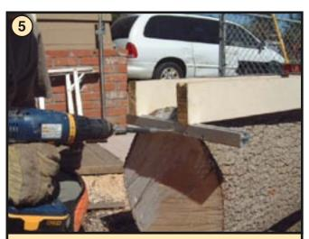
Attach brackets to one end of the log. You may need to drill and toe nail the 2 x 4 to stabilize the guide on the other end.
