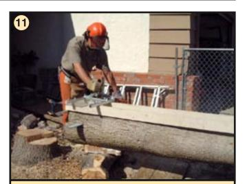
Set mill on guide rails and make your first cut. Push the mill evenly through the wood keeping the mill guides down on the 2 x 4's. Use a small wedge and insert in saw cut when you have cut approximately half of the slab. Keep the mill level when exiting the cut.
