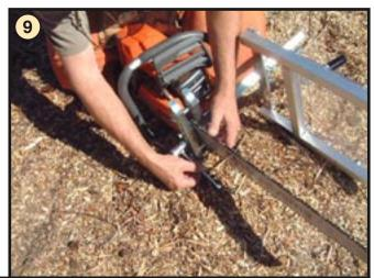
Attach the Small Log Mill to your saw as shown. Make sure clamping olts are equally spaced from the center of the bar. Tighten to 10 to 12 lbs. of torque.
