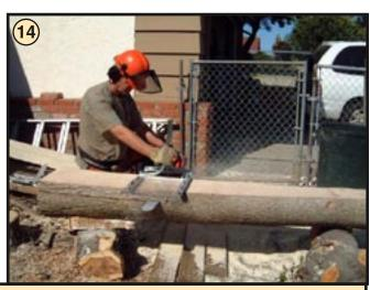
Adjust mill to desired thickness. Proceed with following cuts.
