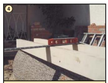
Level guide system in cross diection. If the log tapers from one end to the other and you want to cut down the center of the log, then you may need to raise one end of the guide system up.
