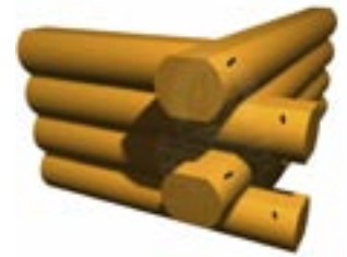
Angled Drill Pattern Near Log Ends (On upper or lower side of logs. Placing on lower side of log will make rods less noticeable.)
