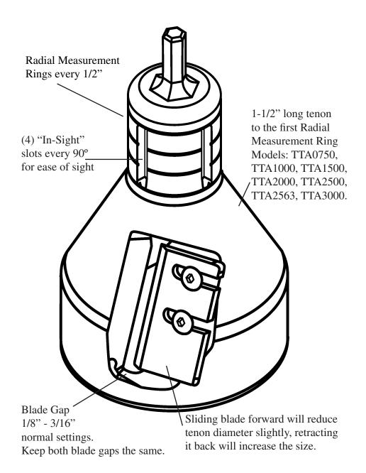
NOTE: *Do Not* slide it back more than 1/4" or it will not cut. Make sure blade is fully exposed.
