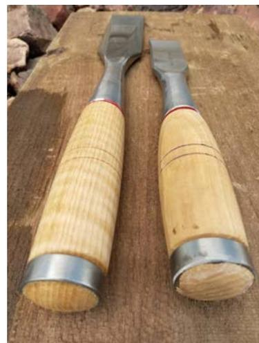
The [Bench Chisels](#) may be used just as hard, and require just as much durability and sharpness. However, because they are used at the 'work bench' they are shorter and easier to handle up close than the Framing Chisels. If you are choosing a chisel for yourself or a friend, be sure to select one designed for the task in mind.
