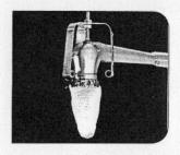
C. Apply a flame to the mantle, but do not turn on the valve until the mantle has burned completely white.
