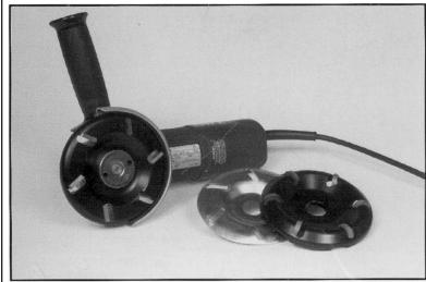
Carbide and steel wheel discs used to trim and shape hooves, woods and plastics.
